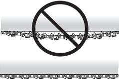
**Keep cutting equipment well lubricated and properly maintained!** A poorly lubricated chain is more likely to break and lead to increased wear on the bar, chain and drive sprocket.
