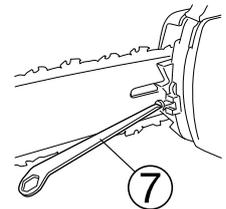
8. Tighten chain firmly but not so hard that it does not turn easily by hand force. Push the button to release the chain brake. To avoid contact between your hands and the chain, use gloves to turn the chain.
