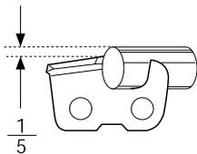
See «Technical Specifications» for the details which apply to your chain. It is very difficult to file a chain saw correctly without the proper aids. We recommend the use of a file guide to ensure maximum cutting efficiency with the least tendency to kickback.
