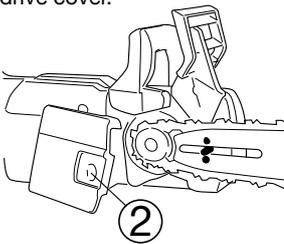
3. Fit the chain around guide bar nose with the top cutters facing forwards.
