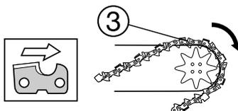
4. Holding the chain over the guide bar nose, position the back end of the guide bar against the drive sprocket at a 45° angle to the power head. Pass the free end of the chain around the drive sprocket, swing the guide bar into place over the mounting bolt and against the power head, and guide the chain into the guide bar groove.
