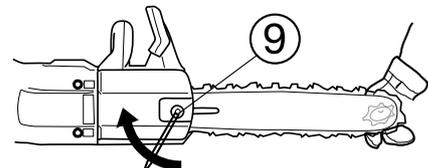
The tension of a new chain must be checked frequently until it is broken in. Continue to check the tension at regular intervals to ensure good performance and a long service life.
