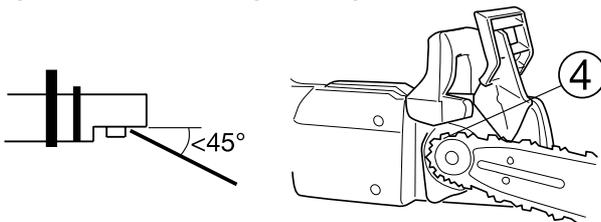
5. Seat the guide bar tensioner pin in its hole in the guide bar.
