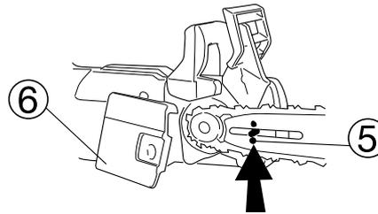
7. Tension the chain by screwing the tensioning screw clockwise using the screwdriver tip on the combination tool.
