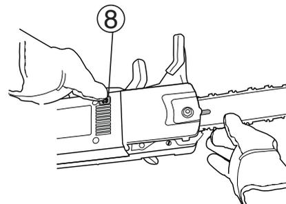
9. Tighten the mounting nut with the combination tool while holding the tip of the guide bar up.
