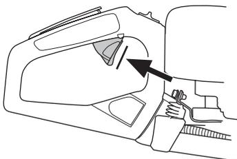
Press the throttle lockout and make sure it returns to its original position when you release it.
