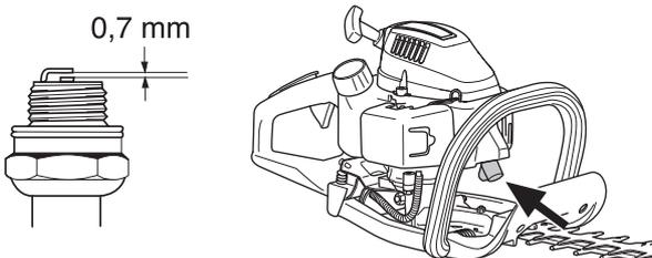
**CAUTION!** Always use the recommended spark plug type! Use of the wrong spark plug can damage the piston/cylinder. Check that the spark plug is fitted with a suppressor.
