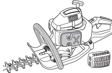
Some mufflers are equipped with a special spark arrestor mesh. If your machine has this type of muffler, you should clean the mesh at least once a week. This is best done with a wire brush.
