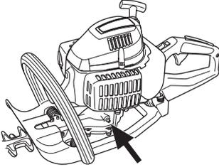
**CAUTION!** The gear housing must not be filled completely with grease. The grease expands as the machine heats up during operation. If the gear housing was completely filled with grease it could damage the seals and lead to leakage of grease.
