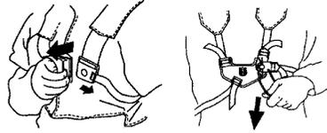
Check that the harness straps are correctly positioned. Once the harness and machine have been adjusted, check that the harness quick release works correctly.
