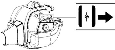
**NOTE:** If engine dies, return blue engine choke lever to the closed position and repeat starting steps.
