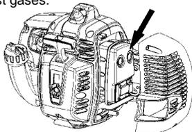
The muffler is designed to reduce the noise level and to direct the exhaust gases away from the operator. The exhaust gases are hot and can contain sparks, which may cause fire if directed against dry and combustible material.
