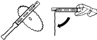
Check the cutting attachment for damage or cracks. A damaged cutting attachment should always be replaced.
