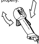
See instructions under the heading Start. Start the machine and apply full throttle. Release the throttle and check that the cutting attachment stops and remains at a standstill. If the cutting attachment rotates with the throttle in the idle position then the carburettor idle setting must be checked. See instructions under the heading Maintenance.
