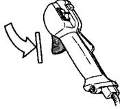
Press the throttle lock-out and make sure it returns to its original position when you release it.
