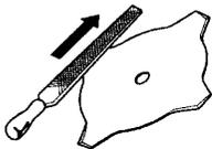
Keep the correct setting on the saw blade! Follow our instructions and use the recommended setting tool. An incorrectly set saw blade increases the risk of jamming and blade thrust, and damage to the saw blade.
