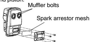
**CAUTION!** Never use a machine that has a faulty or loose muffler. Ensure the muffler bolts are tight.
