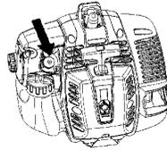
**Choke:** Move the blue engine choke lever over to the closed position.
