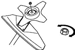
The nylon lining inside the locking nut must not be so worn that you can turn it by hand. The lining should offer a resistance of at least 1.5 Nm. The nut should be replaced after it has been put on approx. 10 times.
