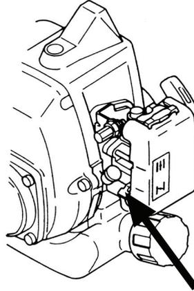
**Start throttle:** Set the throttle to the start position by first pressing the throttle lockout and the throttle trigger, then pressing the start throttle button (A). Then release the throttle lockout and the throttle trigger, followed by the start throttle button. The throttle function is now activated. To return the engine to idle, press the throttle lockout and throttle trigger again.
