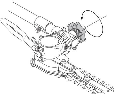
**CAUTION!** When the stop position has been passed the blades are blocked, do not try to cut with the cutting unit in this position.
