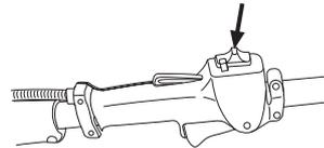
Start the engine and make sure the engine stops when you move the stop switch to the stop setting.
