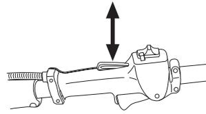
Check that the throttle control and throttle lockout move freely and that the return springs work properly.
