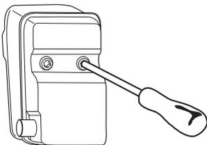
If the muffler on your machine is fitted with a spark arrestor mesh this must be cleaned regularly. A blocked mesh will cause the engine to overheat and may lead to serious damage.
