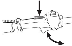
See instructions under the heading Start. Start the hedge trimmer and apply full throttle. Release the throttle trigger and check that the blades stop and remain stationary. If the blades move when the throttle trigger is in the idle position then the carburettor idle setting must be adjusted. See instructions under the heading Maintenance.
